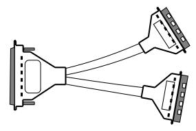
Figure 9–5 shows an HD68 trilink connector (H885-AA), which you may attach to a KZPSA-BB or KZPBA-CB adapter that has its onboard termination removed, an HSZ40 or HSZ50 controller, or the unterminated differential side of a SCSI signal converter.
